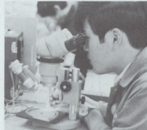
Electric welding of extremely fine resistance wire is performed with care by Masatoshi Ishikawa.
