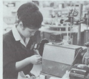
Kimie Kanoh winds transformer coils. Components group also provides printed circuit boards.
